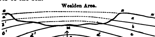
Fig. 4.—Strata diminishing in thickness over the central or Wealden area. a , Upper Chalk; b , Lower Chalk; c , Gault and Lower Greensand; d , Weald clay or Old Wealden land.
